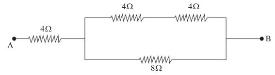
Find out equivalent resistance between the points A and B in the following circuit diagram.
