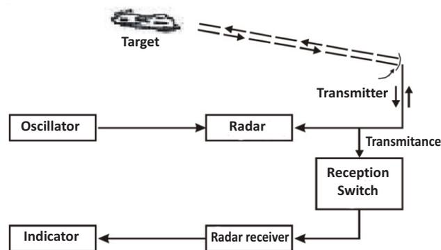
**Fig. 11.11 : Components of a Radar and its functioning**
