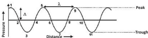
**Fig. 11.5 : Graphical representation of the sound wave**
