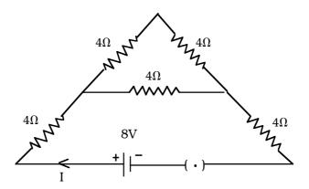
Determine the equivalent resistance and total electric current I passing through the given circuit diagram. 2 + 1 = 3
