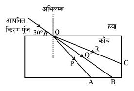
In the given ray diagram write the value of angle of incidence and name of refracted ray.
