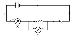
Write Ohm's law. Write name of devices X and Y in the given circuit related to Ohm's Law. 1+1+1=3
